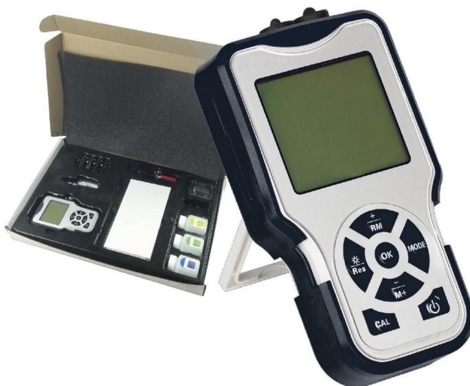
Measure conductivity, TDS, salinity, resistivity, dissolved oxygen and temperature of water solutions and very cost effective.
