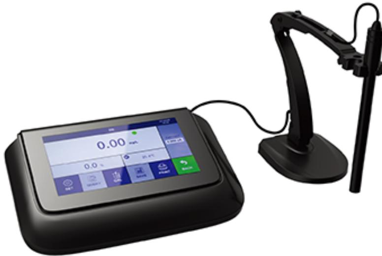
Laboratory bench Dissolved Oxygen meter, which is suitable for aquaculture, water source monitoring, waste water treatment and environmental protection monitoring and other industries, also widely used in education and scientific research fields.
