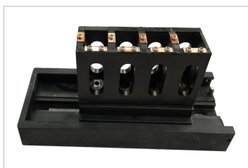
Manual 4-position cell holder
